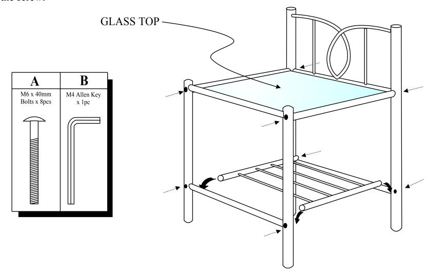
\*\*Periodically check and ensure that all the screw and joint are tight.\*\*
